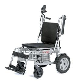
A cross-brace designed folding powered wheelchair with removable footplates, a reclining backrest and twin batteries with a range of up to 24 km. Renowned FreedomChair build quality.
