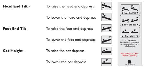
Note: When putting the mattress platform into tilt it is only possible to have one end in tilt at any one time. Before raising one end ensure that the opposite end is fully lowered.
