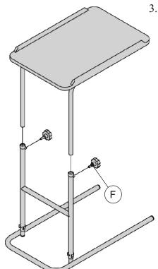
3. Connect the two sections of the table together as shown above. Adjust the table top to the required height and angle. Insert the two handscrews (shown by 'F') in to the receiver in the frame. Secure the table in position by turning two handscrews clockwise until they lock the table tubing in position.
