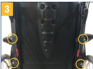
To adjust the backrest height, loosen the 4 hexagon socket screws in the retaining clips and move the backrest into the desired position, then re-tighten screws.
