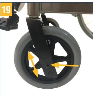
The height of the steering wheels can be changed in three steps.
