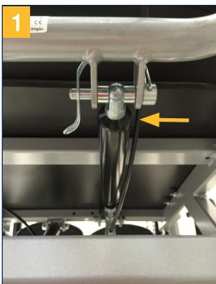
Set the backrest upright and attach the backrest to the frame base using the connecting pin. Push the connecting pin through the slots and secure the pin with the locking clip. Make sure that the pin is locked securely.
