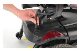
8. Plug the cable from the joystick remote in to the port at the centre of the powerchair base.
