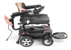
5. Set the arms to the required width then secure by turning the armrest knobs clockwise.
