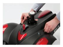
2. Connect the battery pack. Refit the shroud and tighten the two knobs to secure.
