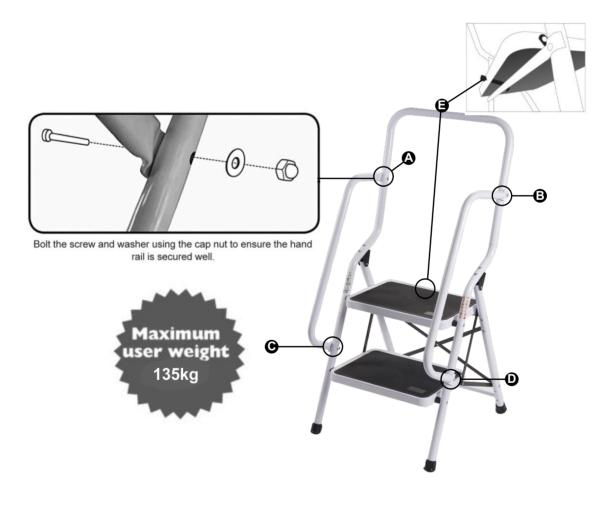
**Note:** The step ladder will support itself by spreading its weight and balancing through a scissor movement.
