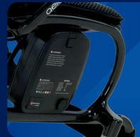
Air travel safe, lightweight lithium battery with off board charging
